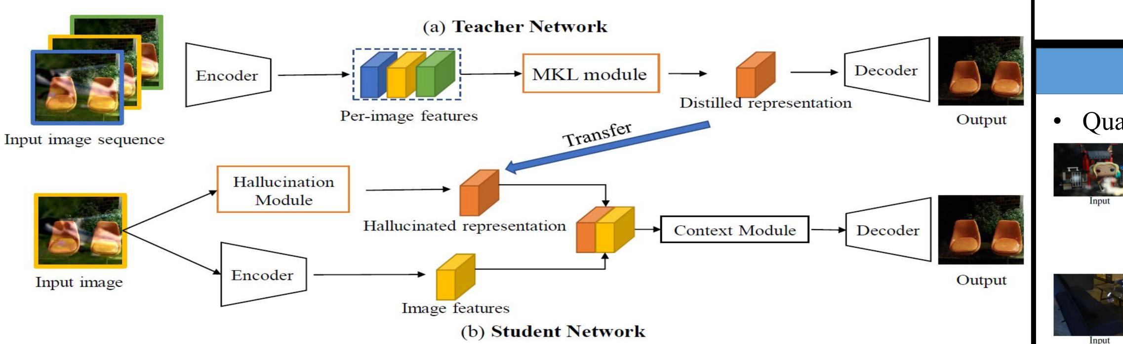
Overview of our learning framework. (a) Teacher Network. The input is a multi-view image sequence and the output is the estimated transmission layer of the middle image of the input sequence. (b) Student Network. The input is a single image (or the middle image of the sequence during training) and the output is the estimated transmission image.
